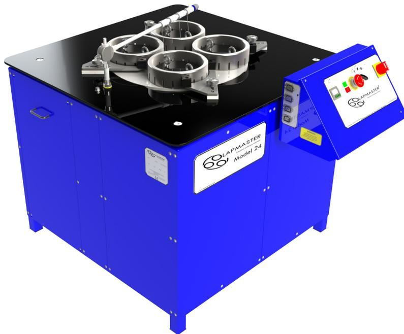
The Lapmaster Wolters Model 24 is the smallest floor standing lapping machine in the range and is ideal for engineering workshops, where flatness and finish are of prime importance. It is equipped with a 610mm diameter serrated lap plate, manufactured from Grade 300 grey cast iron to ISO 185(2005) as standard. Other plates can be supplied on request.
